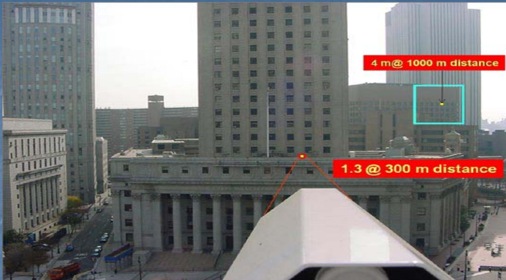
Due to the fact that the beam divergence angles in optical wireless systems are very narrow, the FSO community typically uses milliradian as measure for beam divergence. 1 Radiant (rad)=57.3 degrees or 1 milli radiant (mrad)=0.0573 degrees. In other words, the divergence angle in mrad roughly corresponds to the beam diameter at a distance of 1 kilometer from the originating source.
