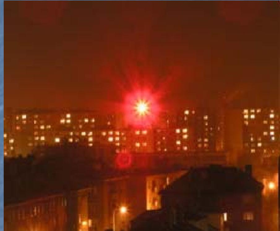
single high-output LED with a 13cm glass lens. The beam is about 4 meters wide in 1km.
