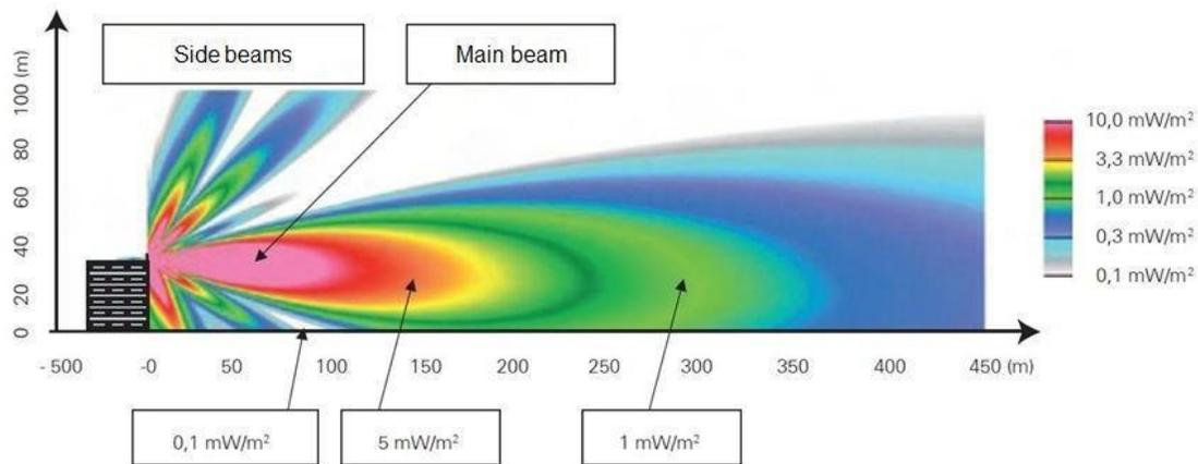
The simulation to the left shows the radiated power distribution of a mobile phone base station antenna in space. Besides the main beam, which covers long-range areas, side beams are emitted at certain angles to cover short range areas.
